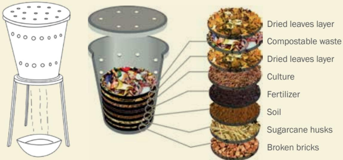
Material needed: Plastic or Earthen pot with holes at the bottom, Broken bricks, Soil, Fertilizer (micro-organisms or commercially available EM culture), Dried leaves and compostable waste, A small vessel to collect the seepage, Tripod stand, Lid.
